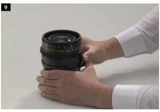
Put the ring back on the lens. The desired scale unit is now visible in the window of the scale reading.
