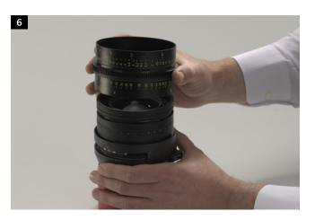
Lift the scale ring and take it off the lens.
