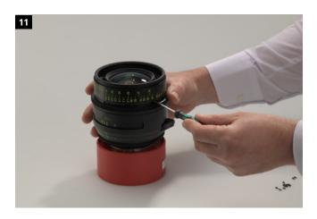
Lift the scale ring slightly up as soon as you can see the holes and tighten the nine T4 Torx screws under use of the T4 screwdriver (0,15Nm).
