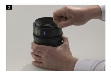
Remove the flexible rubber ring at the front side of the lens.
