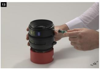
Tighten the six Torx screws under use of the T4 Torx screwdriver. (0,15Nm).
