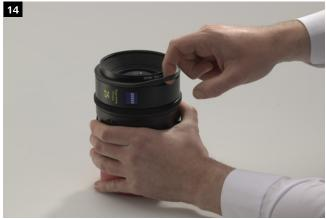
Mount the rubber ring with the thin side on top on the compendium ring.
