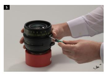
Loosen the nine screws by using the T4 Torx Screwdriver.
